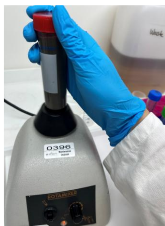
Figure 2 Vortexing soil and acetonitrile
