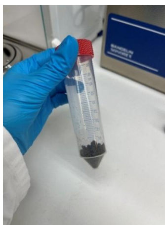
Figure 1 5 g soil sample in 50 mL centrifuge tube
