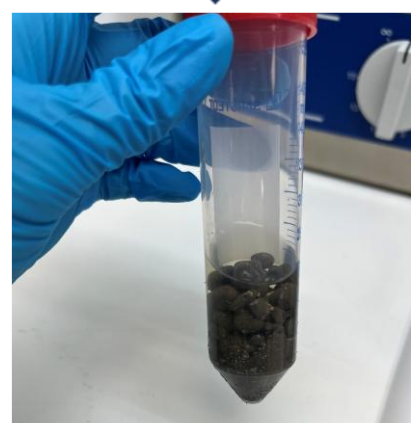
Figure 4 Salts added and vortexed
