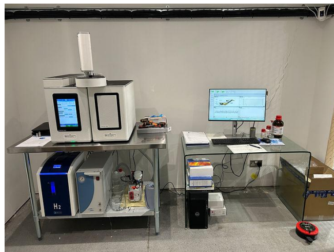
Figure 1 SCION Helium Free GC-MS installed at customer site with FDGSI hydrogen generator (picture provided by SCION Instruments UK distributor CE Instruments). [2]
