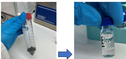
Figure 2 From soil sample to clear sample, suitable for GC analysis
