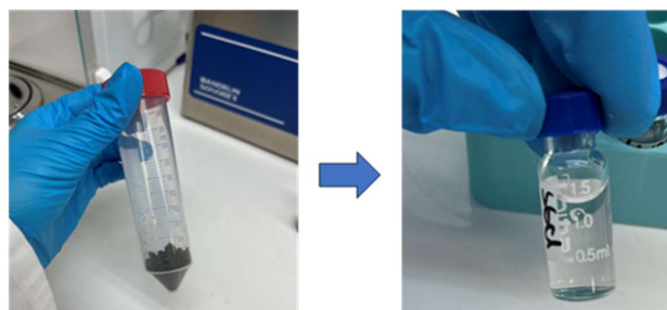
Figure 3 From soil sample to clear sample, suitable for GC analysis
