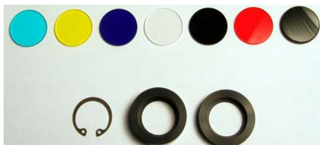
Figure 2 PFPD band pass optical filters
