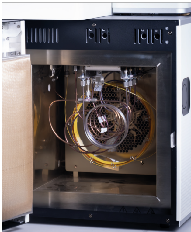
Figure 7: 'Traditional' RGA with all columns mounted in oven.
