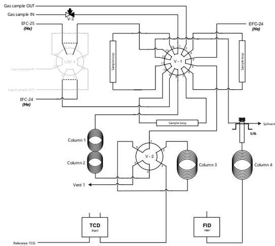
Figure 1: Flow diagram Natural Gas System C
