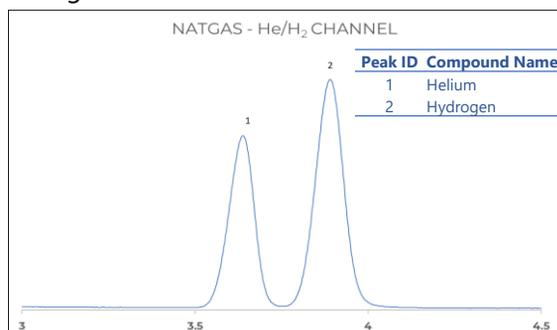
**Figure 4: Helium and Hydrogen analysis on TCD channel**
