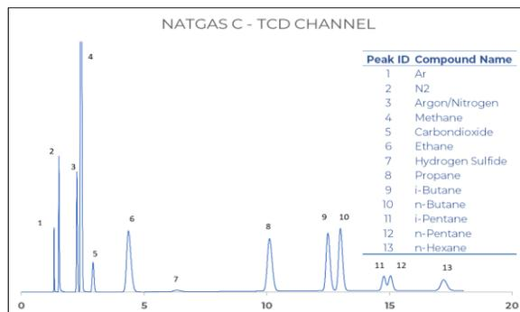
Figure 2: Permanent gases on TCD channel
