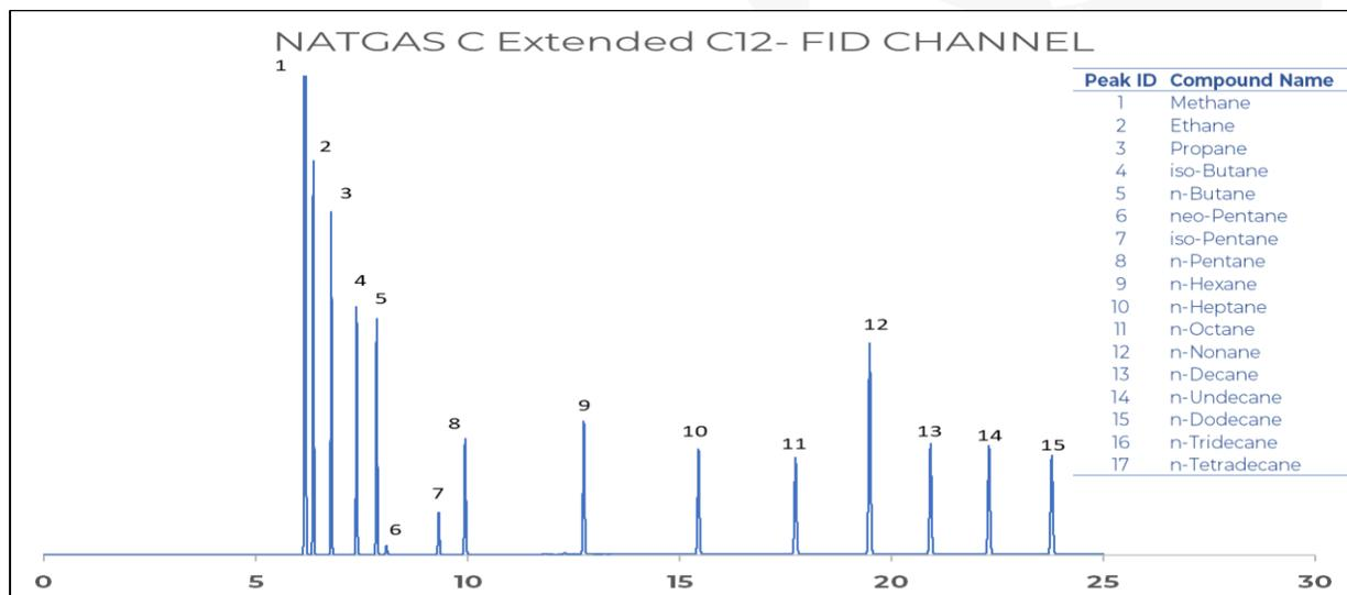
**Figure 3: Extended hydrocarbon analysis on FID channel**
