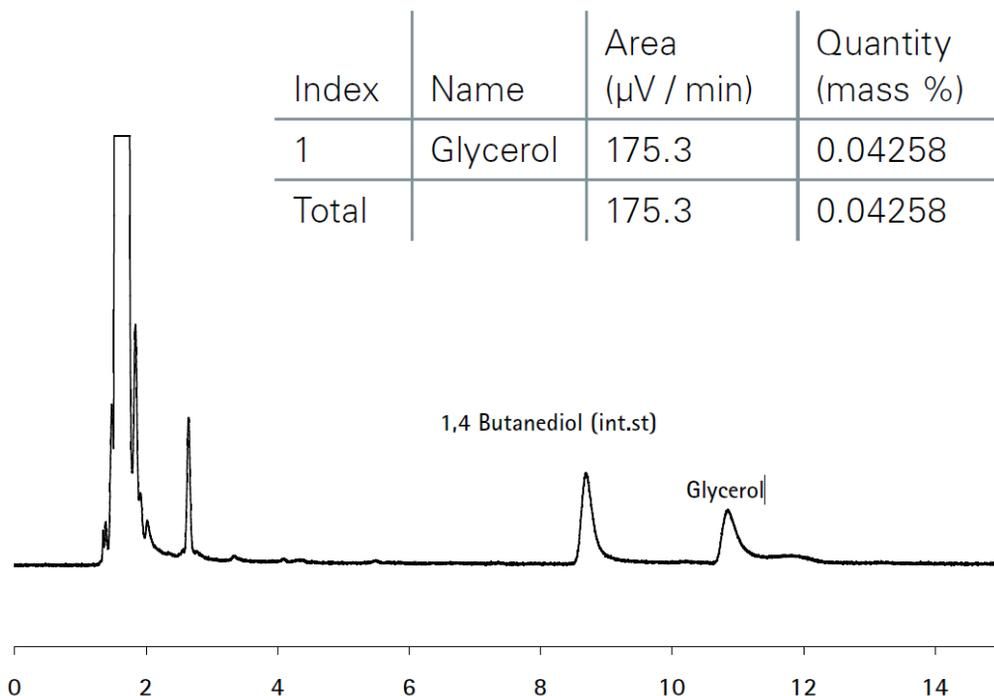
Fig. 1 Biodiesel Chromatogram
