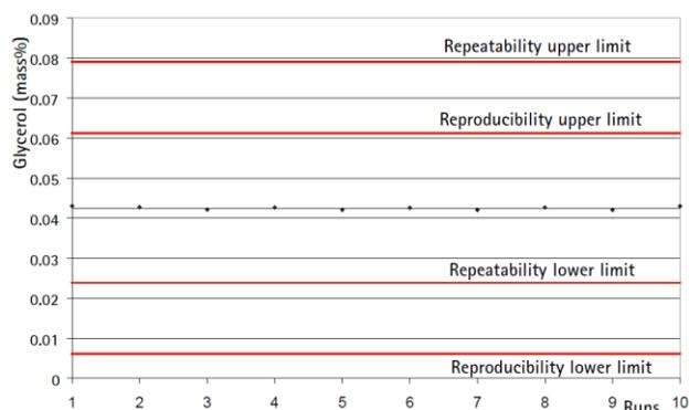
**Fig. 2 - Repeatability based on 10 runs. Red lines indicate the maximum and minimum variation limits of the method.**
