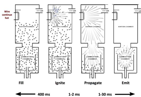
**Fig 1.** Schematic operation of the PFPD
