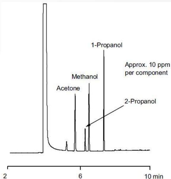
Figure 6. Analysis of Oxygenates on GC-2
