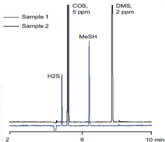
Figure 8. Analysis of Sulphur Components on GC-2
