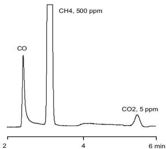
Figure 4. Analysis of CO, CH4 and CO2 on GC-1
