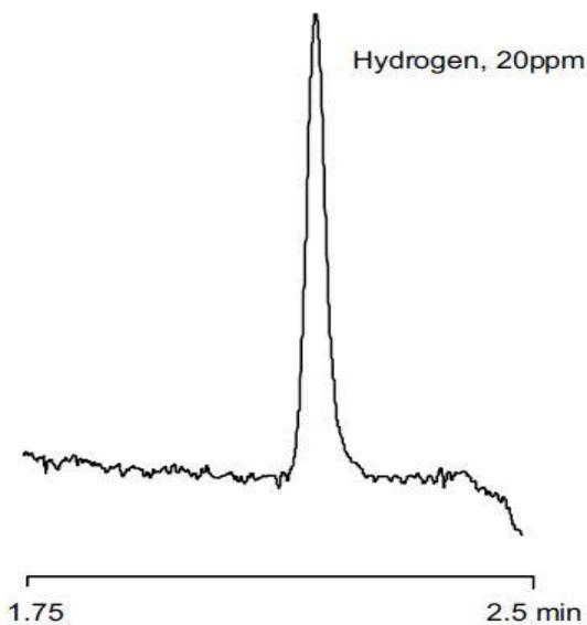
Figure 3. Hydrogen Analysis on GC-1
