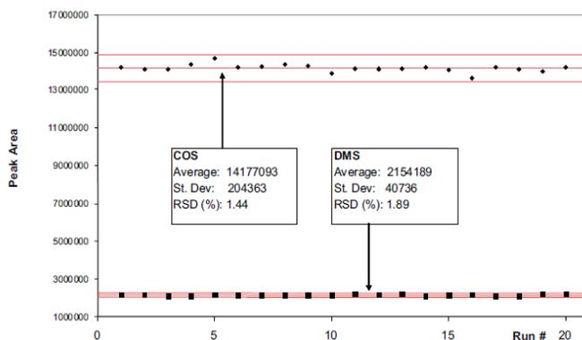
Figure 15. Repeatability data of Sulphur Components with 5% Variation Limits
