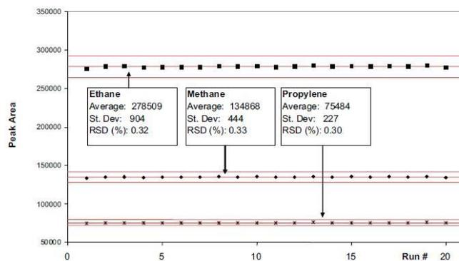
Figure 14. Repeatability data of Light Hydrocarbons with 5% Variation Limits
