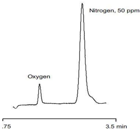
Figure 5. Analysis of O2 and N2 on GC-1
