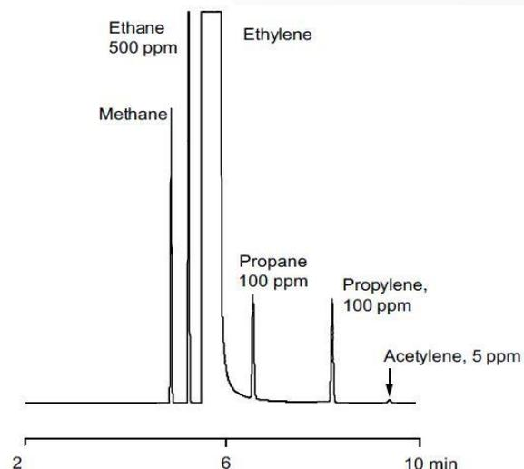
Figure 7. Analysis of Light Hydrocarbons on GC-2
